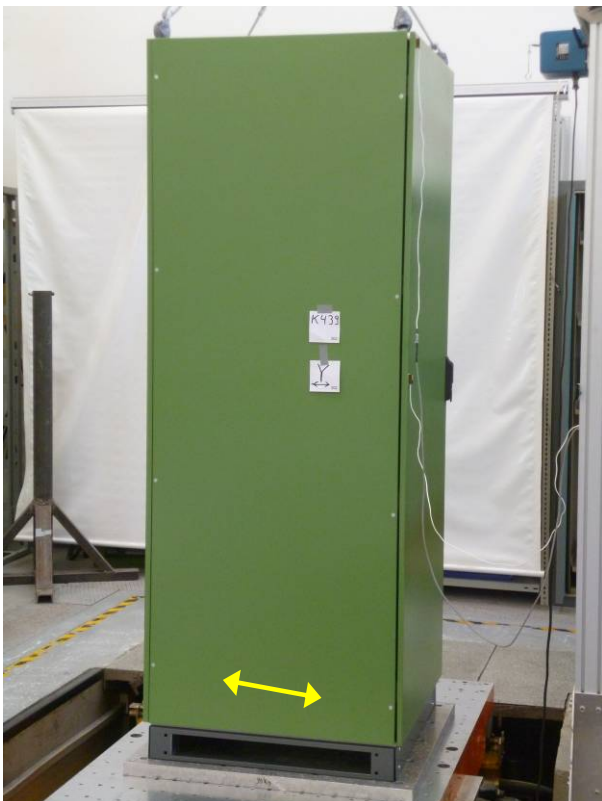
Pic. 14 Mounting of EUT for Y-axis test
