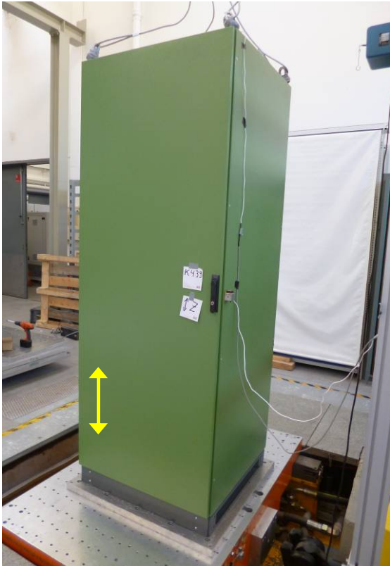
Pic. 12 Mounting of EUT for Z-axis test
