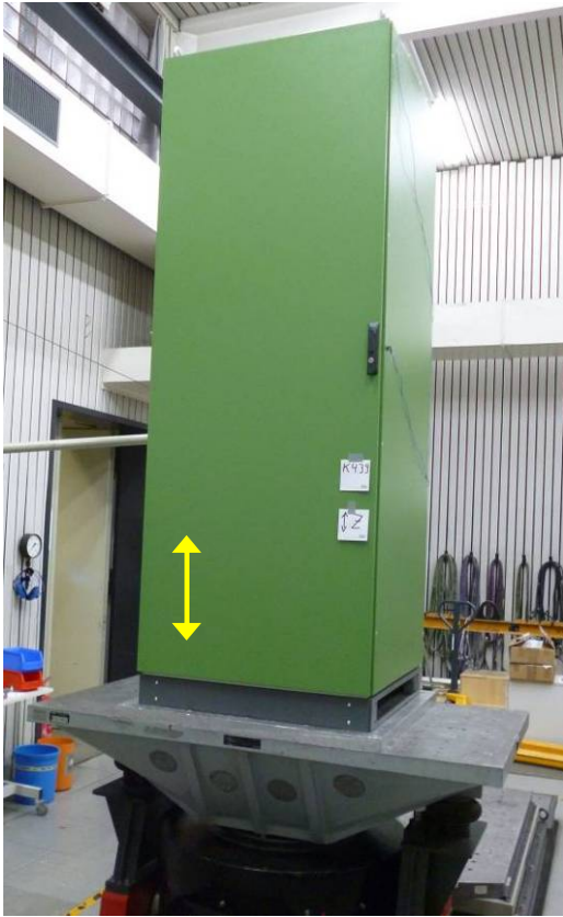
Pic. 5 Mounting of EUT for Z-axis test
