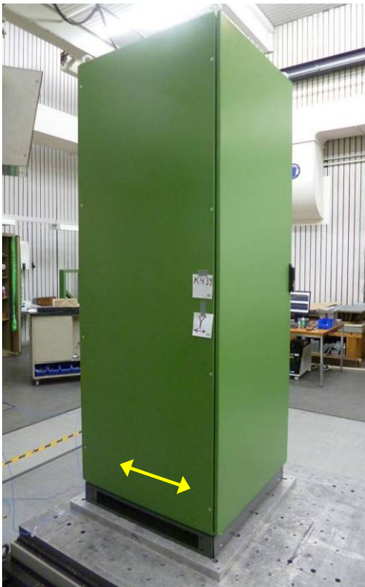
Pic. 7 Mounting of EUT for Y-axis test
