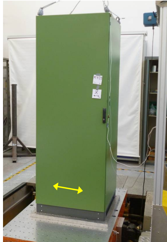
Pic. 13 Mounting of EUT for X-axis test
