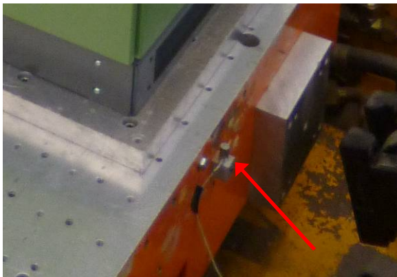
Pic. 8 Measuring point for time history at earthquake table
